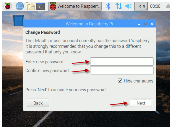
Figure 24 Creating a Password for the Raspberry Pi
